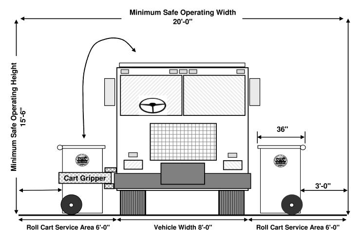
Note: The attached diagram is designed to provide a general reference for safe operating distances for typical automated sideloading refuse collection vehicles. Some service locations may have unique characteristics that may require additional evaluation to allow for roll cart service.
